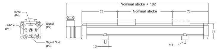
4 pins connector (View toward sensor pins)
