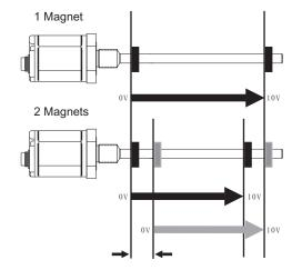
When using dual magnets, there is a minimum distance of 76mm need to be kept in between.
