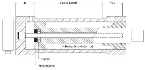
16C series is design for use in extreme harsh environments with high contamination and presence of dust. Sensing element is protected by fully enclosed stainless steel case with IP68 protection rating. It is completely dustproof and resistant to harsh salty air, flooding and powerful water jetting. This unique product is perfect for use in harsh indoor applications and severe outdoor environments.
