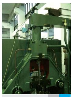
Hot chamber die-cast machine used Germanjet 17 series
