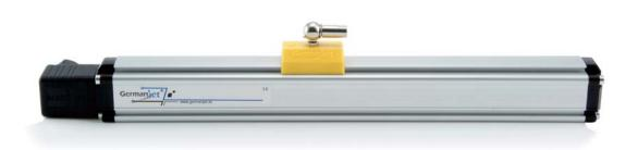
The fundamental principle of the magnetostrictive transducer is by analyzing the feedback sonic wave induced by an interaction of two magnetic fields. The first magnetic field is produced by the moveable magnetic cursor which attached at the moving component of a machine. The second field is generated by the pulse initiator. After the two magnetic fields interact, a sonic wave is induced and detected by the sonic wave analyzer.
