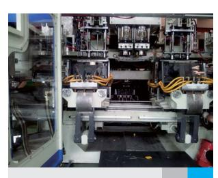
Fast mold shifting at blow molding machine
