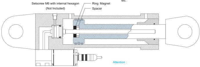
The ring magnet should not intouch with the sensor rod.
