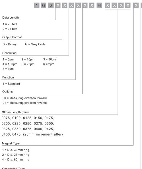
Remark: Direction forward means position reading become larger while magnet move away from electronic carriage. Direction backward means position reading become smaller while magnet move away from electronic
