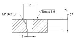
Installation hole must be perpendicular with mounting surface and center with sensor rod.
